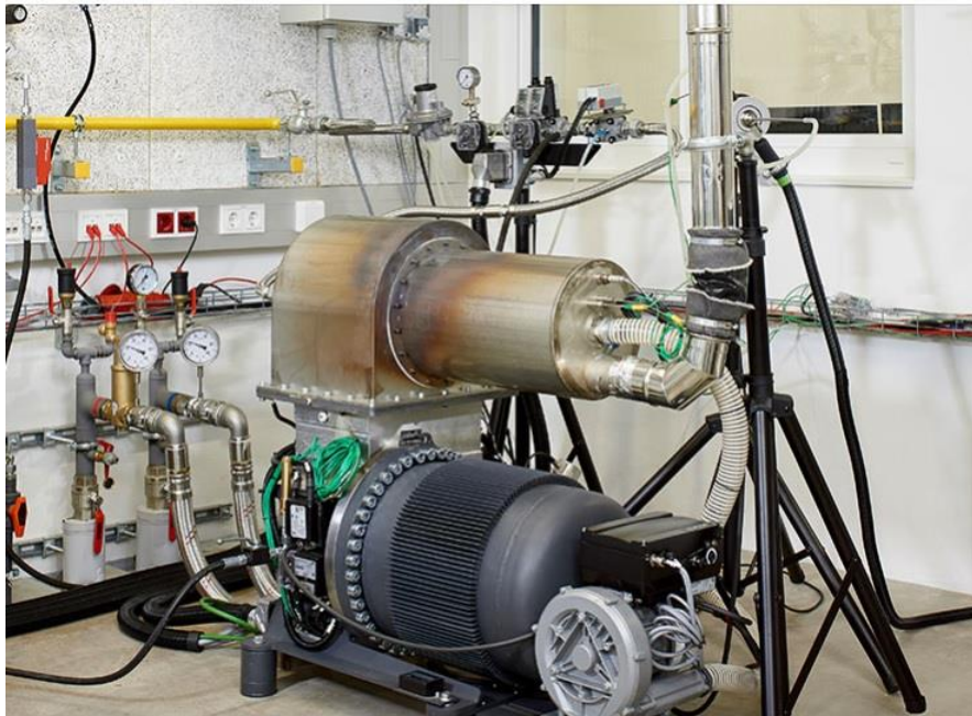
Figure 171: Photo of the 8 kW alphagamma® Stirling engine model G600i ("Frauscher thermal motors," 2019).
