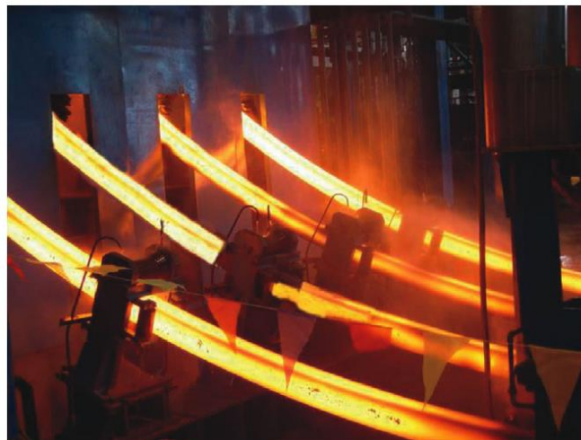
Figure 196: Steel billets after continuous casting (Utlü, Paralı, & Gültekin, 2018).
