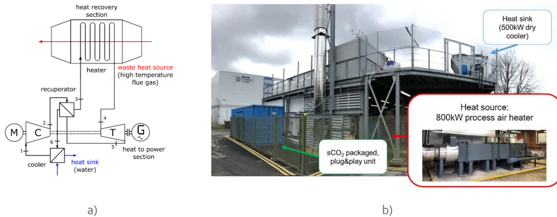
Figure 151: sCO 2 power cycle demonstrator for industrial WHR built at Brunel University within the I-Therm H2020 project (M. Marchionni, Saravi, Bianchi, & Tassou, 2019).
