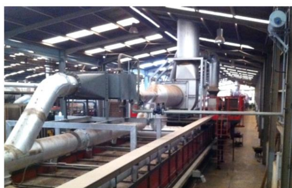
Figure 111: WHR from ceramic kilns: a) Schematic of a tile tunnel kiln showing the exhaust gases and the hot cooling air as potential heat sources for the ORC (Casci et al., 1981); b) photo of the recovery facility implemented in Spain composed by a recuperator (located in the bypass line of the cooling air) and a heat transfer loop with thermal oil (Navarro-Esbrí et al., 2013).
