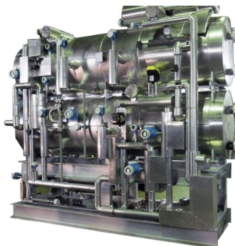
Figure 226: Picture of the 200 kW AHT developed within the EU project Indus3ES (Indus3Es H2020, 2019).
