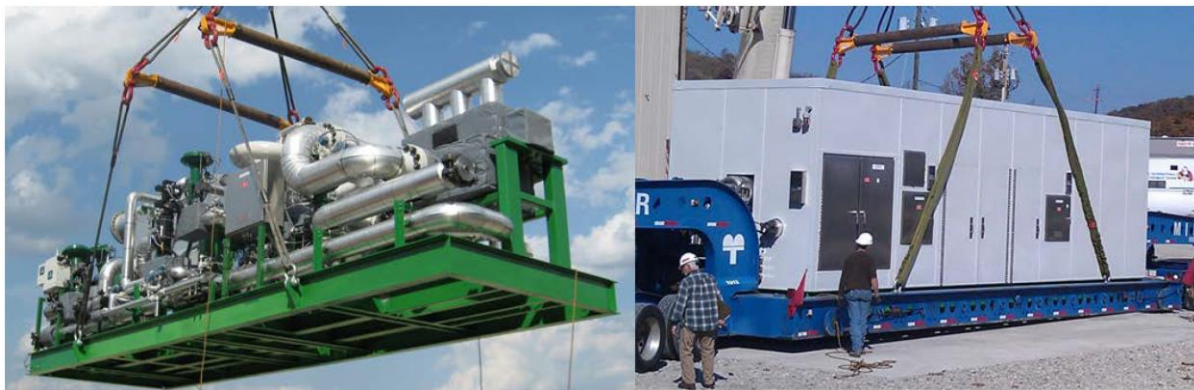
Figure 149: 6-8 MW advanced sCO 2 heat engine (EPS100), process and power skids (T. J. Held, 2015).
