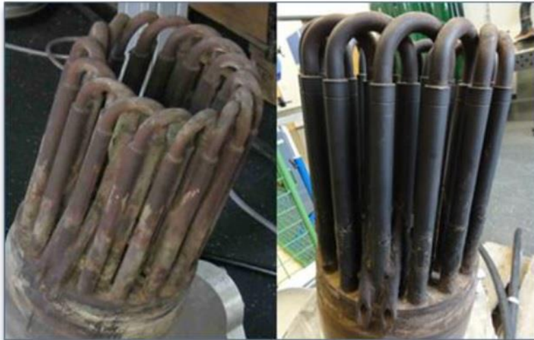
Figure 168: HE surfaces of the Stirling engine heater before and after the tests (Schneider et al., 2018).
