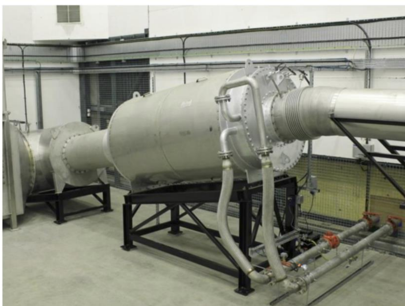
Figure 77: Gas-to-oil HPHE ("Econotherm," 2020).
