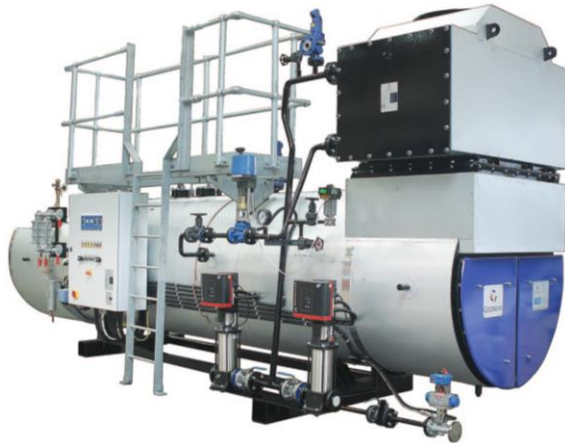
Figure 46: Fire tube WHB with a capacity of 3000 kg/h and a thermal power output of 2 MW for various industrial applications (WHR from engines, thermal oxidizers, gasifiers, etc.) ("Cochran UK," 2019).
